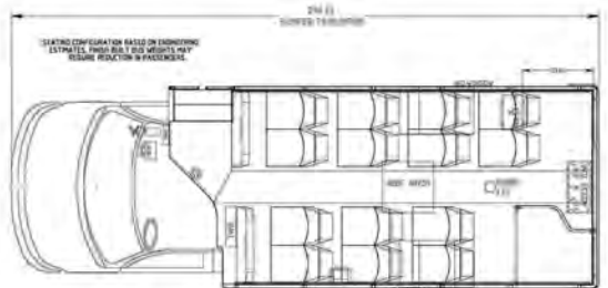
01500 MASTERS TRANSPORTATION SEATING PLAN 14 Passengers 2 36 inch ACTIVITY W/C Seats at 28 inch Hip to Knee 3 35 inch ACTIVITY LH Seats at 28 inch Hip to Knee
